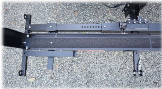
(INSTALL LEFT PAN OVER RIGHT PAN)
